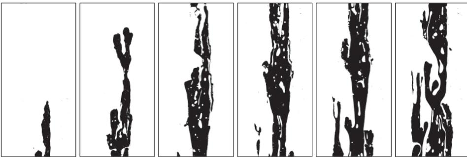
Figura 4.122: Solução de goma xantana 0,40% deslocando óleo mineral –  $\dot{\gamma} = 240,19$  1/s;  $u^* = \dot{\gamma}^* = 9,576$ ;  $\eta^* = 0,187$ ;  $\dot{m} = 1,040$  g/s;  $Re = 0,707$ ;  $We = 4,726.10^{-3}$ ;  $Ca = 1,635.10^{-2}$ ;  $T = 24^\circ C$ ;  $\varepsilon = 28,370\%$ , *Fingers*.
