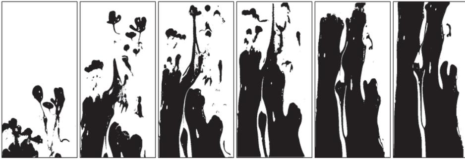
Figura 4.67: Solução de poliacrilamida 0,25% deslocando óleo mineral –  $\dot{\gamma} = 303,9781/s$ ;  $u^* = \dot{\gamma}^* = 12,48$ ;  $\eta^* = 0,165$ ;  $\dot{m} = 1,412 \text{ g/s}$ ;  $Re = 0,951$ ;  $We = 8,615 \cdot 10^{-6}$ ;  $Ca = 1,462 \cdot 10^{-2}$ ;  $T = 22^\circ C$ ;  $\varepsilon = 63,940\%$ , *Fingers*.
