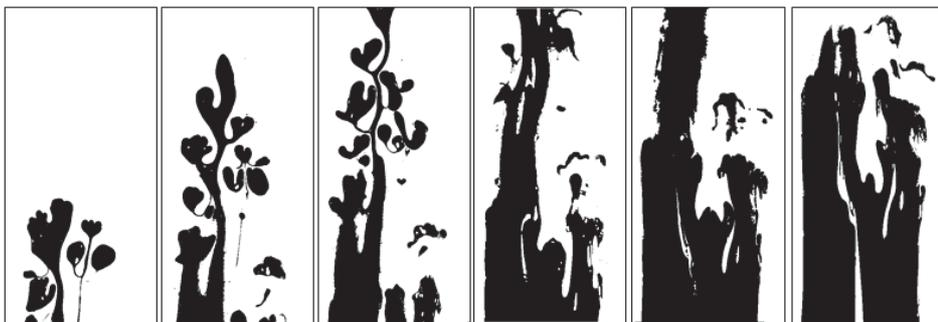
Figura 4.69: Solução de poliacrilamida 0,25% deslocando óleo mineral –  $\dot{\gamma} = 355,4471/s$ ;  $u^* = \dot{\gamma}^* = 14,591$ ;  $\eta^* = 0,148$ ;  $\dot{m} = 1,651 \text{ g/s}$ ;  $Re = 1,243$ ;  $We = 1,178 \cdot 10^{-5}$ ;  $Ca = 1,307 \cdot 10^{-2}$ ;  $T = 22^\circ C$ ;  $\varepsilon = 56,198\%$ , *Fingers*.
