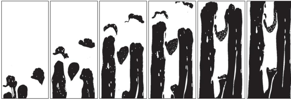
Figura 4.64: Solução de poliacrilamida 0,25% deslocando óleo mineral –  $\dot{\gamma} = 186,5201/s$ ;  $u^* = \dot{\gamma}^* = 6,944$ ;  $\eta^* = 0,251$ ;  $\dot{m} = 0,867$  g/s;  $Re = 0,412$ ;  $We = 3,244.10^{-6}$ ;  $Ca = 2,271.10^{-2}$ ;  $T = 23^\circ C$ ;  $\varepsilon = 65,960\%$ , *Fingers*.
