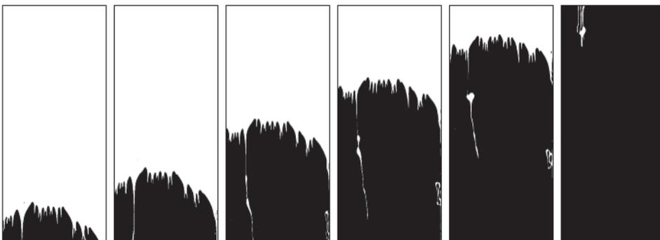
Figura 4.42: Óleo mineral deslocando solução de poliacrilamida 0,25% –  $\dot{\gamma} = 462,862$  1/s;  $u^* = \dot{\gamma}^* = 22,952$ ;  $\eta^* = 0,107$ ;  $\dot{m} = 2,470$  g/s;  $Re = 0,182$ ;  $We = 1,739 \cdot 10^{-2}$ ;  $Ca = 8,476 \cdot 10^{-2}$ ;  $T = 20^\circ C$ ;  $\varepsilon = 99,526\%$ , *Plug*.
