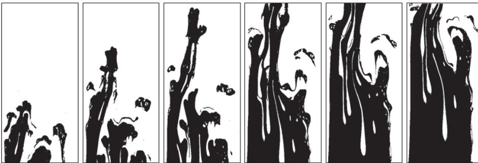
Figura 4.68: Solução de poliacrilamida 0,25% deslocando óleo mineral –  $\dot{\gamma} = 311,3391/s$ ;  $u^* = \dot{\gamma}^* = 14,062$ ;  $\eta^* = 0,152$ ;  $\dot{m} = 1,446 \text{ g/s}$ ;  $Re = 0,990$ ;  $We = 9,039 \cdot 10^{-6}$ ;  $Ca = 1,313 \cdot 10^{-2}$ ;  $T = 21^\circ C$ ;  $\varepsilon = 63,940\%$ , *Fingers*.
