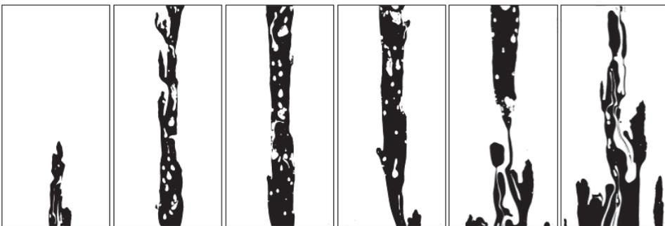
Figura 4.125: Solução de goma xantana 0,40% deslocando óleo mineral –  $\dot{\gamma} = 326,364$  1/s;  $u^* = \dot{\gamma}^* = 14,322$ ;  $\eta^* = 0,138$ ;  $\dot{m} = 1,413$  g/s;  $Re = 1,207$ ;  $We = 8,726 \cdot 10^{-3}$ ;  $Ca = 1,183 \cdot 10^{-2}$ ;  $T = 23^\circ C$ ;  $\varepsilon = 23,568\%$ , *Fingers*.
