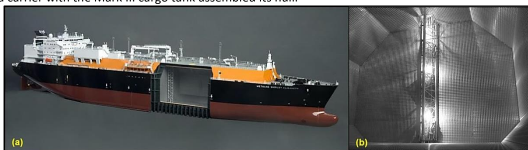
Figure 28 - (a) LNG carrier with a Mark III cargo tank in the hull (b) Internal view of the Mark III cargo tank.
