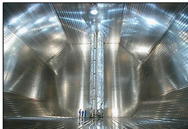
Figure 13 – Double membrane cargo tank with CS1 system.
