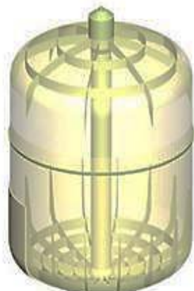
Figure 14 – Schematic drawing of the independent cargo tank Type B
