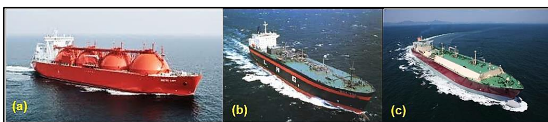
Figure 7: (a) LNGCs with spherical, (b) prismatic and (c) membrane cargo tanks.
