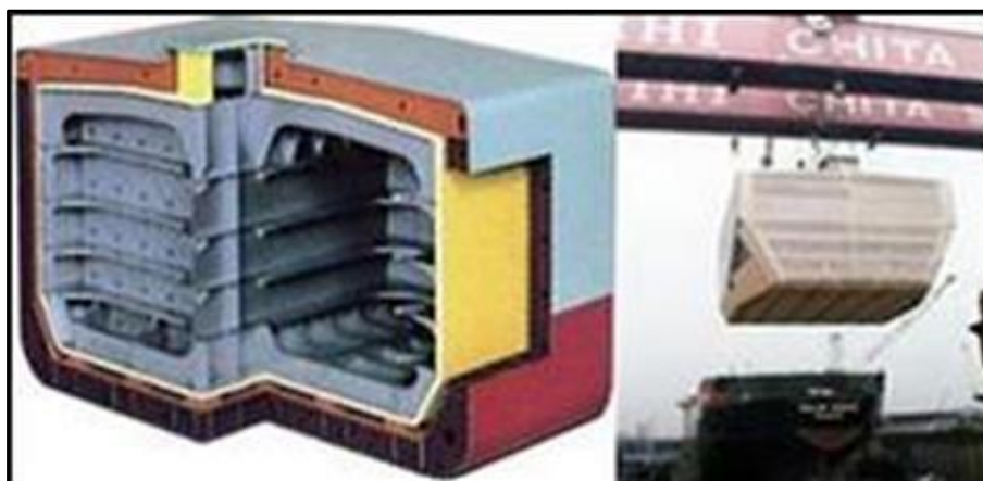
Figure 10 – Cross section and hook up of a prismatic tank type SPB
