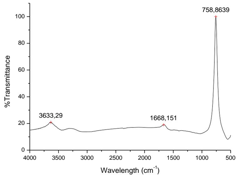
Figure 31 - FTIR spectra of hematite after interaction with *Rhodococcus ruber* biomass and principal %transmittance peaks
