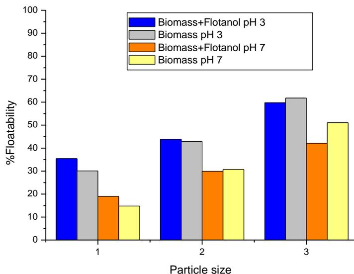
Figure 37 - Effect of Flotanol in the bioflotation of hematite with *Rhodococcus ruber* in function of pH and particle size (biomass concentration  $0,15 \text{ g.L}^{-1}$ )
