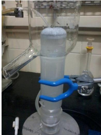
Figure 36 – Hematite bioflotation using *Rhodococcus ruber* biomass in a Partridge-Smith flotation cell (pH 3; biomass concentration: 0,15 g.L<sup>-1</sup>; using flotanol).
