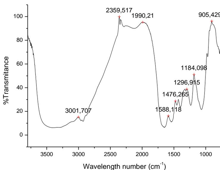
Figure 29 – FTIR spectra for *Rhodococcus ruber* biomass and principal %transmittance peaks
