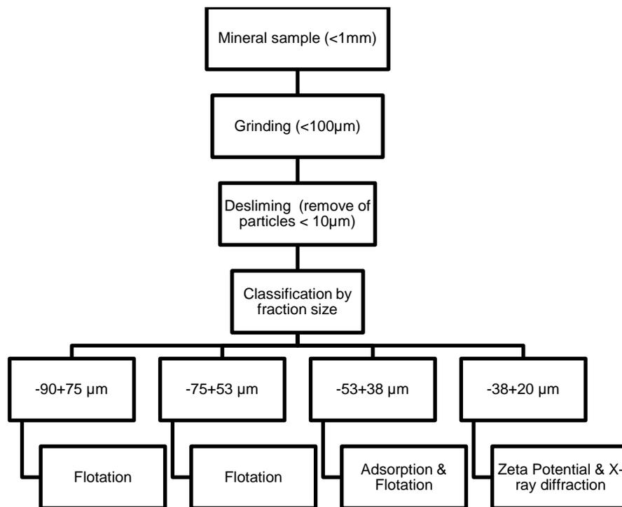
Figure 18 - Flowchart of hematite pre-treatment and characterization
