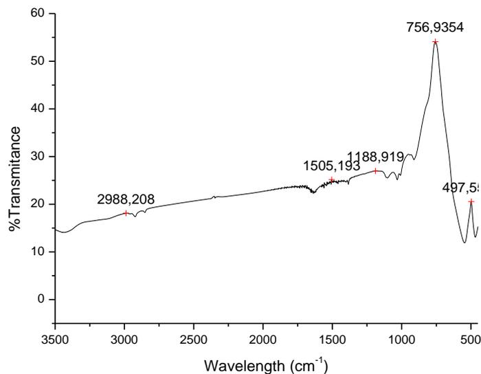
Figure 30 – FTIR spectra of the hematite sample and principal %transmittance peaks
