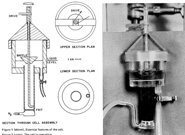
Figure 32 - Partridge-Smith flotation cell used for the flotation of the hematite-dodecylamine-starch system (Partridge-Smith, 1971)
