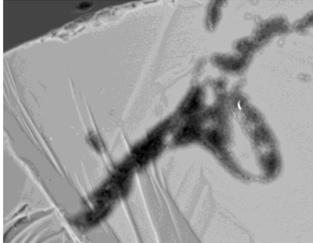
Figure 40 - Scanning electron micrograph of hematite clean sample after interaction with *Rhodococcus ruber* biomass, for particle size range -53+38 $\mu\text{m}$  (Magnification x3000)
