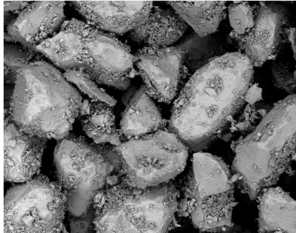
Figure 19 – Scanning electron micrograph of hematite sample after grinding (no ultrafine particles removal) for particle size range  $-53+38\mu\text{m}$  (Magnification x200)
