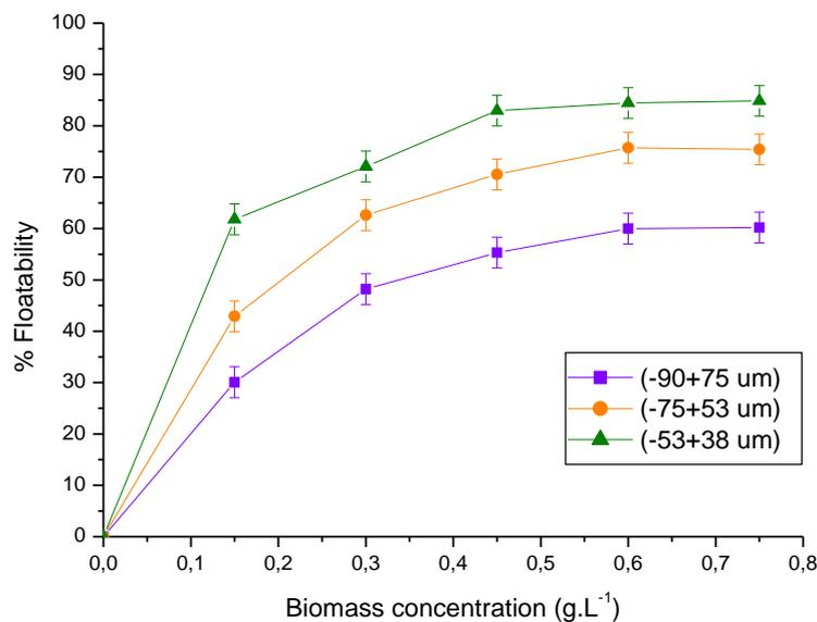
Figure 33 - Hematite microflotation as function of biomass concentration (particle size range: 90-75 $\mu\text{m}$ , 75-53  $\mu\text{m}$  and 53-38 $\mu\text{m}$ ; flotation time: 5min; pH 3)
