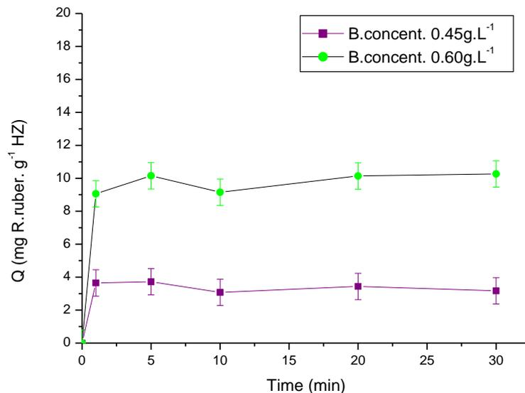
Figure 27 - Adsorption measurements for *Rhodococcus ruber* adsorb onto hematite surface in function of the conditioning time (biomass concentration: 0,45 g.L<sup>-1</sup> and 0,60 g.L<sup>-1</sup>; particle size range: -53+38  $\mu$ m)
