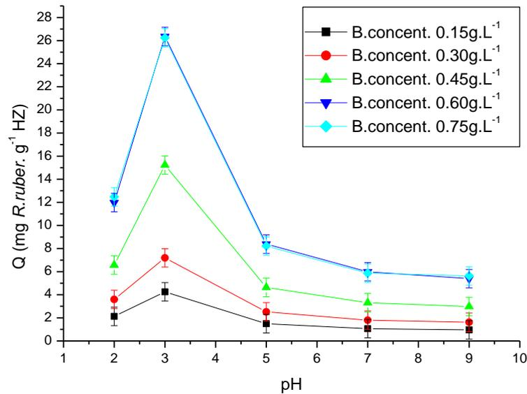
Figure 28 - Adsorption measurements for *Rhodococcus ruber* adsorb onto hematite surface in function of pH (conditioning time: 5min; particle size range: -53+38  $\mu\text{m}$ )
