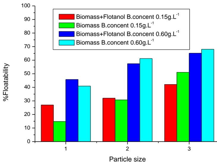
Figure 38 - Effect of Flotanol in the bioflotation of hematite with *Rhodococcus ruber* in function of biomass concentration and particle size
