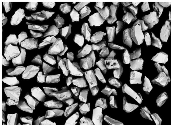
Figure 39 – Scanning electron micrograph of hematite clean sample after interaction with *Rhodococcus ruber* biomass, for particle size range -53+38 $\mu\text{m}$  (Magnification x120)
