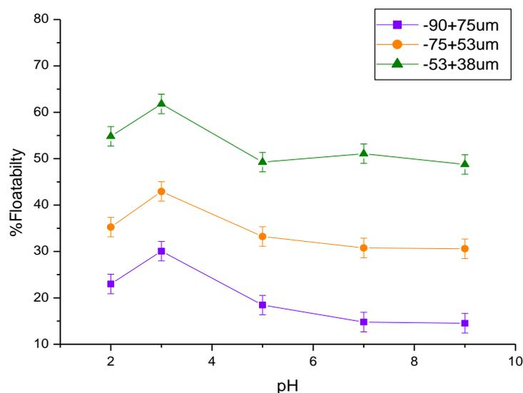
Figure 34 – Hematite microflotation as function of pH (particle size range: 90-75µm, 75-53 µm and 53-38µm; flotation time: 5 min; biomass concentration:  $0,15 \text{ g.L}^{-1}$ )
