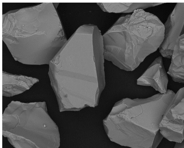
Figure 20 - Scanning electron micrograph of hematite sample after desliming for particle size range  $-53+38\mu\text{m}$  (Magnification x200)
