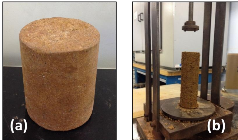
Figure 3.17 - Specimen preparation: (a) Compacted cylinder and (b) clayey soil after the shaping.
