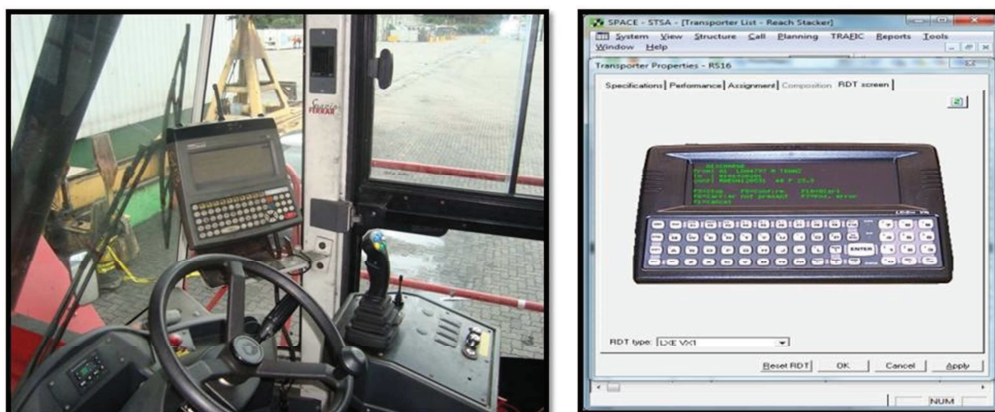
Figura 6 – Vehicle Mount Terminal
