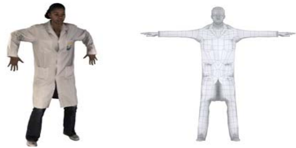
Figure 5: Original “High Polygons” 3D model and the final low polygon mesh.
