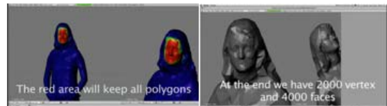
Figure 10: Interactive polygon reduction allowing details on desired places (Wartman, 2008)
