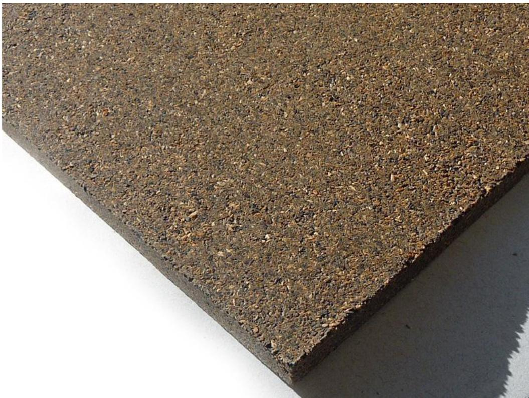
Figura 46 – Placa 70/30 –  $900\text{kg/m}^3$  -  $300 \times 200 \times 10\text{mm}$ . Fonte: Anne Mello, 2012.
