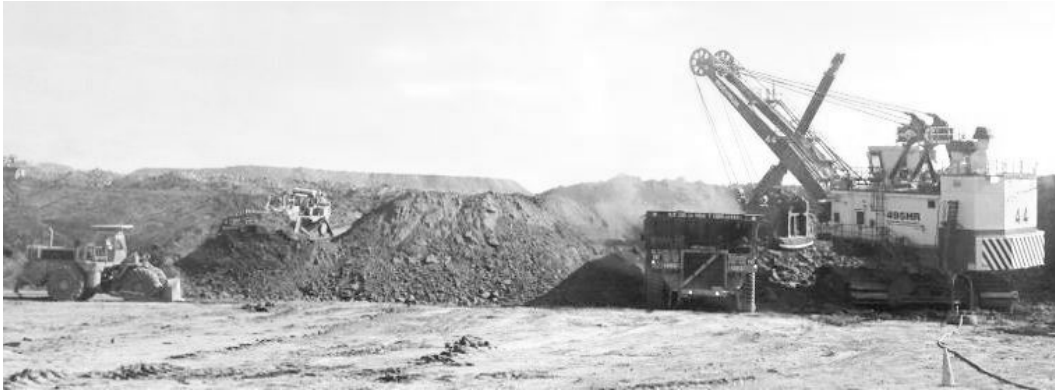
Figure III.1: Synchronized operation of mine vehicles. Vehicles from left to right: Rubber Tire Dozer , Bulldozer , Truck , Shovel
