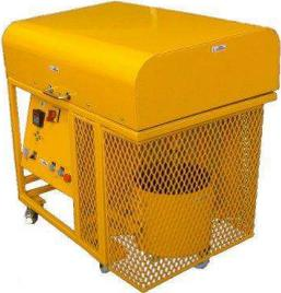
A photograph of a yellow two-point workability test apparatus, which is used to measure the flow and spreading of concrete under a specific load.                                                                                                                                                                                                                                                         | Viscosidade e tensão de escoamento |
