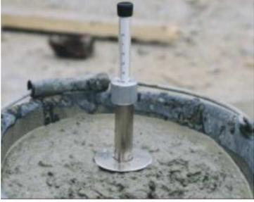
A photograph showing a K-slump test apparatus. It consists of a cylindrical metal rod with a flat base, used to measure the consistency of fresh concrete by determining the depth of the slump.                                                                                                                                                                                                            | Tensão de escoamento               |
