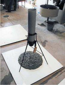
A photograph of the Orimet apparatus, a mechanical device used to measure the plastic viscosity of concrete by rotating a spindle in a sample.                                                                                                                                                                                                                                                            | Viscosidade plástica               |
