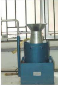
A photograph of a Vê-Be consistency meter, a mechanical device used to measure the plastic viscosity of concrete by rotating a spindle in a sample.                                                                                                                                                                                                                                                         | Viscosidade plástica               |
