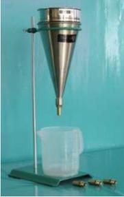
A photograph of a Marsh cone apparatus, which is a funnel-shaped device used to measure the flow time of a concrete sample under a specific load to determine its plastic viscosity.                                                                                                                                                                                                                       | Viscosidade plástica               |
