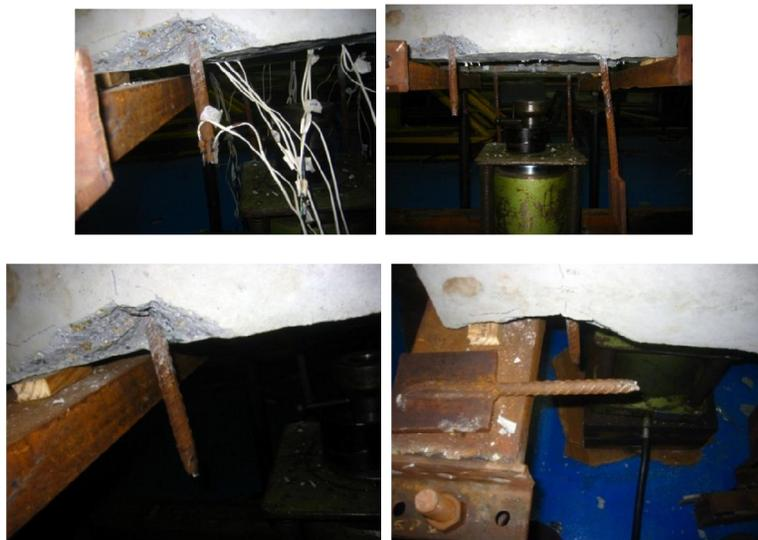
Figura 5.45 – Ruptura do Pull-out PO 0.1
