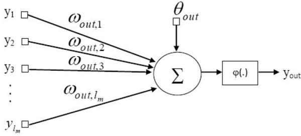
Fig. 5. Output Neuron of the NSP's neural network with  $l_m$  neurons in the hidden layer
