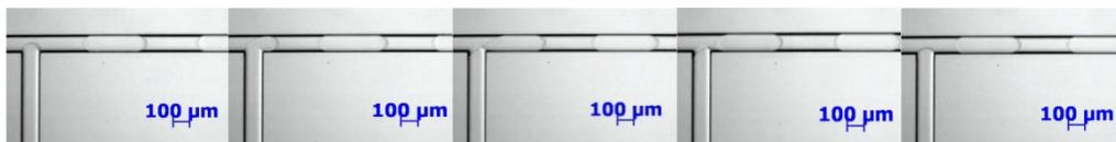
Figura 4.6: Formação de gota observada no sistema N°4 para  $Q_d=0.05$  ml/h e  $Q_c=0.05$  ml/h ( $\mu_d=3.4$  mPa.s,  $\mu_c=12.47$  mPa.s,  $\sigma=9.3$  mN/m,  $\mu_d/\mu_c=0.27$ ).  $L=390.83$   $\mu\text{m}$ ,  $L_{\text{mín}}=379.24$   $\mu\text{m}$ ,  $L_{\text{máx}}=403.75$   $\mu\text{m}$ .  $\Delta t=60$  ms.
