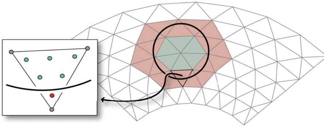
Figure 4.3: Gaussian quadrature: only Gaussian points lying inside the particles  $p_i$  are used to integrate over the domain  $\Omega_{p_i}$ .
