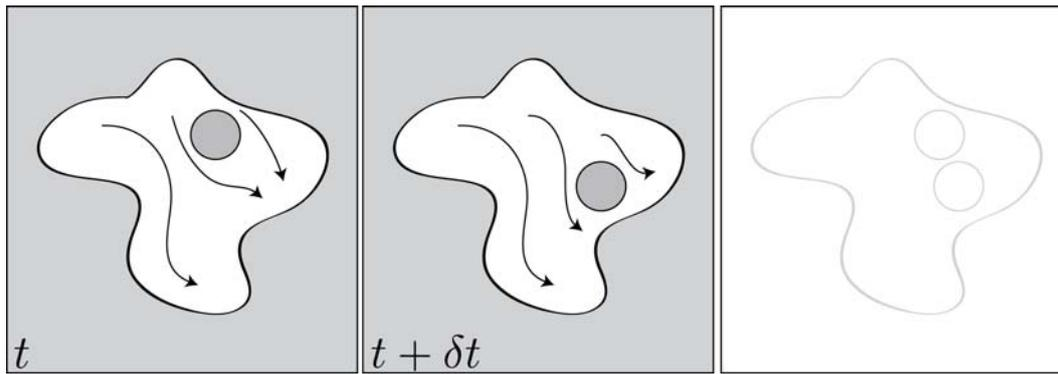
Figure 4.1: Fictitious domain: a problem defined on a geometrically complex domain (white region on the first two pictures), extended to a larger and simpler fictitious domain (white region on the last image).
