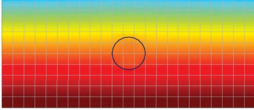
Figure 4.2: Hydrostatic pressure profile obtained by our formulation, using the gravity force on the  $\vec{u}$  momentum.
