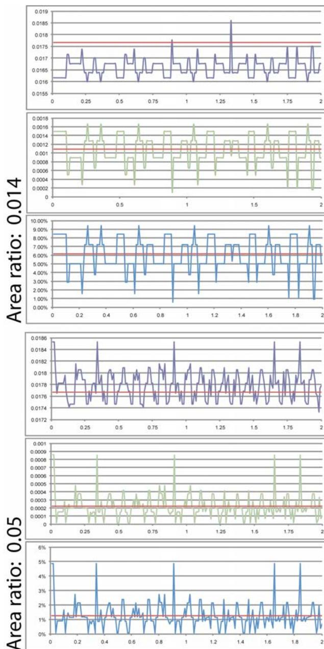
Figure 4.4: Gaussian quadrature: variation of the area of a particle during the simulation time. The first graphs show the results obtained using an area ration 0.014, and the last ones a ration 0.05. In each case, we show the approximated area, the absolute error and the percentage of the analytical area that is neglected by the approximation.
