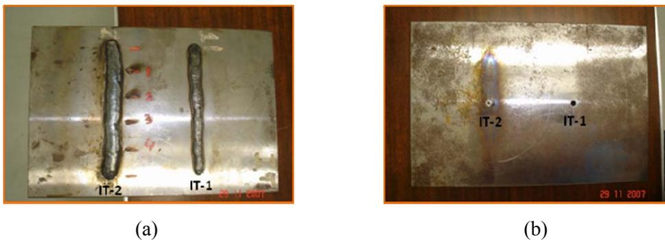
Figura 44: Soldas com arame tubular (a) IT-1 e (b) IT-2.
