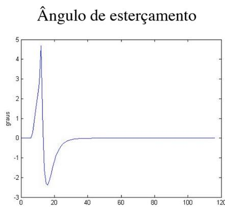
Figura 67: Ângulo de esterçamento - Pólos em  $-2, -3, -4-0.5i, -4+0.5i$ .
