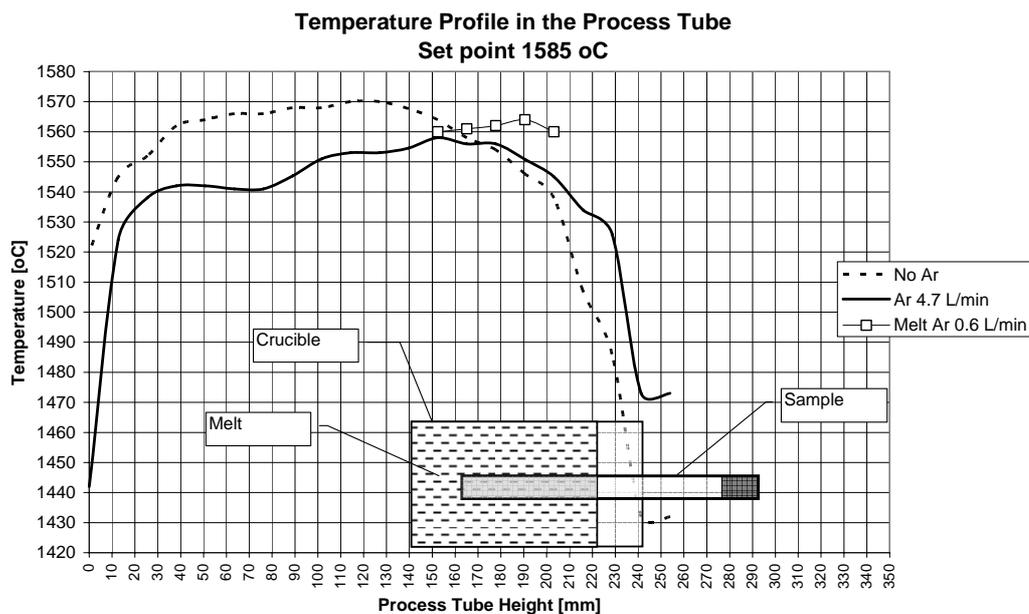
Figure 62 - Temperature profile measured with type B thermocouple at the gas phase in the process tube and in the melt.
