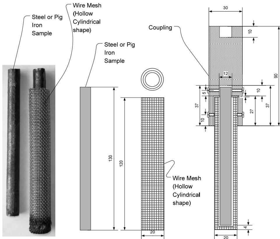
Figure 63 – Steel and pig iron cylindrical samples wrapped up in steel mesh, simulating composed charges.
