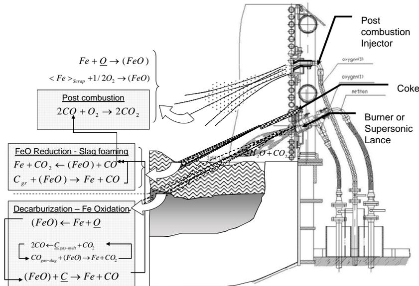
Figure 57 - Example of different oxy-gas-coke injector's applications in EAF
